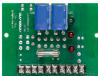
Power supply for AC-225, provides 12 VDC, 2A and 12 VDC, 3 A power outputs and 13.8 VDC for backup battery charging of up to 7 Ah
