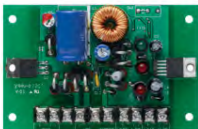
Power supply for AC-215, provides 12 VDC, 0.5 A and 12 VDC, 1.5 A power outputs and 13.8 VDC for backup battery charging of up to 7 Ah
