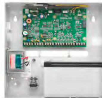
Hardwire Alarm Control panel
